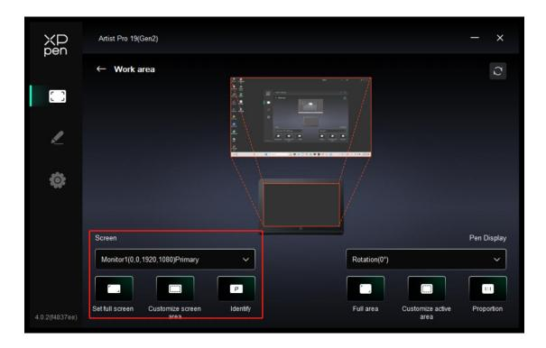
You can set the mapping between the display area of the current monitor and the device.
